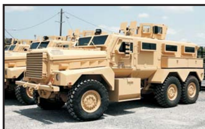
MRAP CAT II Cougars are converted into Joint EOD Rapid Response Vehicles (JERRV) with the primary role of supporting Explosive Ordnance Disposal Specialists by neutralizing Improvised Explosive Devices (IED), mines and other ordnance.
